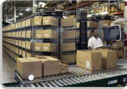
Often used in integrated workstations of carousels called a "pod." This allows an operator to pick from one active carousel while the others are pre-positioning to be picked the moment the operator is ready.
